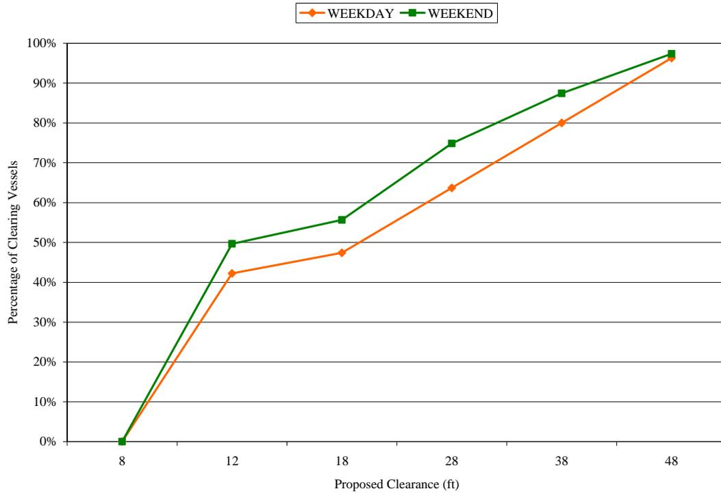
**Figure 5 - Percentage of Vessels Clearing vs. Closed Clearance**
